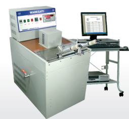
Oxidation Stability By Rotating Pressure Vessel Method (RPVOT)
