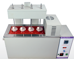
Rust Preventing Characteristics
