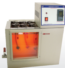
Kinematic Viscosity Bath (For 0.01°C Resolution & Accuracy)
