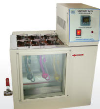
Kinematic Viscosity Bath (For 0.1°C Resolution & Accuracy)
